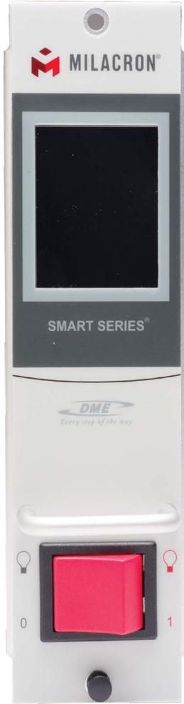
The TSM15 Smart Series Module has a color touch screen digital display providing readouts for Actual Temperature, Current Mode, Percentage Power and Current Reading. Closed-loop, fuzzy logic PID control, and auto-tuning of PID parameters provide precise control even under the most adverse processing conditions.
