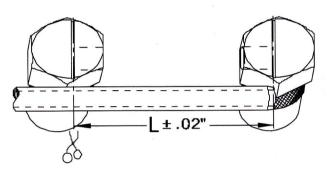
L = Length of cut tube from center of groove to center of groove
