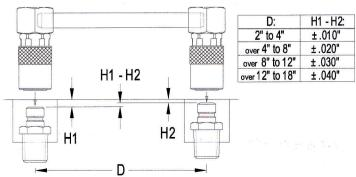
H1 - H2 is the allowable difference in installed height from the edge of the mold to the neighboring plugs.
