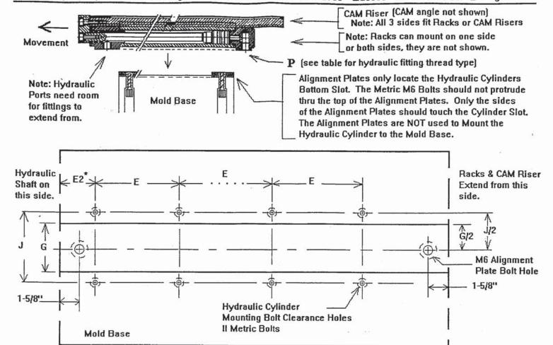
\*-Note: Use E1 value instead of E2 if Hydraulic Cylinder Ports face the side instead of staight down
