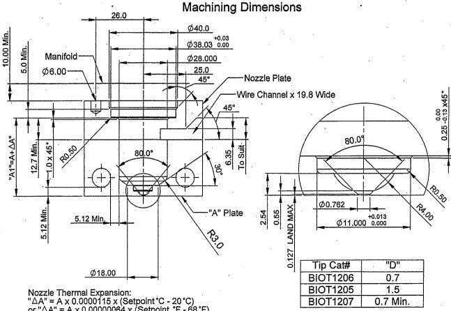
Nozzle Thermal Expansion: " $\Delta A$ " = A x 0.0000115 x (Setpoint °C - 20 °C) or " $\Delta A$ " = A x 0.00000064 x (Setpoint °F - 68 °F)
