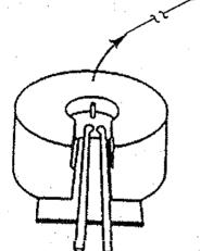
Hold new thermocouple parallel to length of probe. Move thermocouple so there is a "X" inch gap between its tip and the tip of the probe. Mark the thermocouple with a felt tip pen where it would be fully inserted into the probe.
