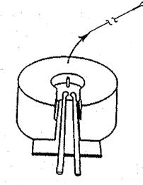
Hold new thermocouple parallel to length of probe. Move thermocouple so there is a "X" inch gap between its tip and the tip of the probe. Mark the thermocouple with a felt tip pen where it would be fully inserted into the probe.
