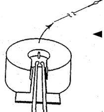
3 Remove thermocouple with long nose pliers, grasping the thermocouple 1/8" from the thermocouple well and remove slowly and carefully.
