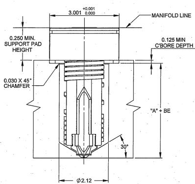
NOTE: Before installing a Point Gate Nozzle, it is important to take the nozzle's expansion factor into consideration. For best results, please follow the information below.
