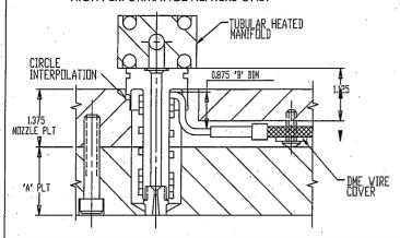
SECTION SHOWING NOZZLE BODY KEYED AND WIRESLOT FOR 1.875 NOZZLE PLATE FOR FRONT LOAD SCH2xxx SQ. COIL HEATERS ONLY
