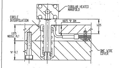
SECTION SHOWING NOZZLE BODY KEYED AND WIRE SLOT FOR 1.875 "A" PLATE FOR FRONT LOAD SCH2xxx SQ. COIL HEATERS ONLY
