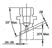
Nozzle body head must be keyed to prevent body from turning when tip is installed into body. Customer to torque (30  $\pm 5$  Ft Lbs) tip into shank of nozzle body in mold three times to set tip before marking the runner or angle on the tip. This will ensure that the tip will line up after runner or angle is machined onto tip. Customer may madhine relief on Extended Sprue Gate Tips and Extended Point Gate Tips for molding heat sensitive or engineering grade materials. (see drawings above)
