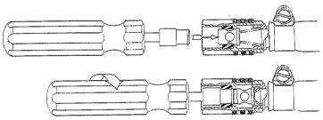
3. Remove tool and seal from socket. (If seal is not completely captured by tool it may remain partially lodged in socket. Seal pick provided can be used to remove seal if this occurs.)
